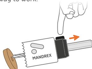
2 REMOVE THE CORE WITH ONE "CLICK"
